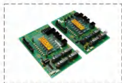
MC24A MC23A Fujitec elevator pcb
