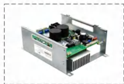
LRU-403(ACD4-MR) Otis elevator inverter
