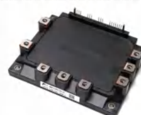
7MBP150RA120-05 Fuji elevator module
