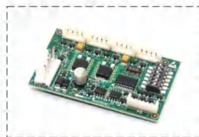
RS14 Otis elevator pcb board
