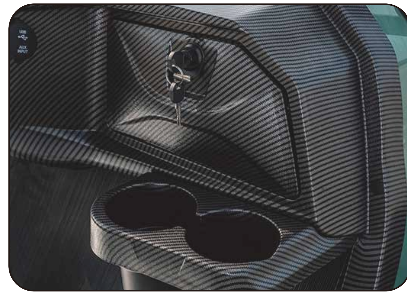
Water transfer printing instrument panel (with leather grain)
