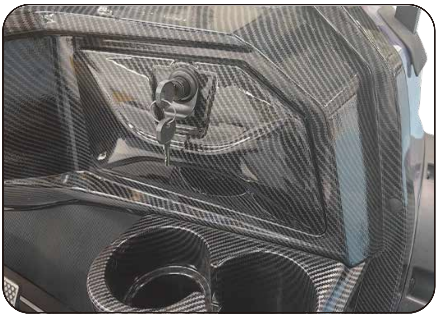
transfer printing instrument panel (without leather grain)
