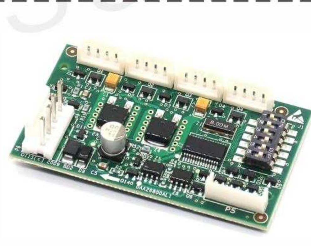
RS14 Otis elevator pcb board
