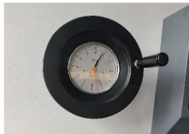
Cutting blade clearance adjustment hand wheel
