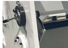
Cutting blade clearance manual adjustment
