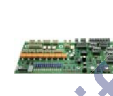
Elevator board Schindler ID.NR.591534 UP001030
