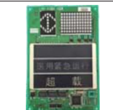
Elevator board Mitsubishi GPS-3 LHD-650A UP002598
