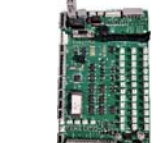
Elevator board ThyssenKrupp UCC CMC3 UP003179
