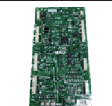
Elevator board Mitsubishi LHD-730AG43 UP000822
