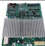
Elevator board Mitsubishi JCI-D1S UP002464
