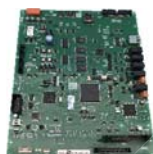
Elevator board Mitsubishi P203769B000G02 UP000812
