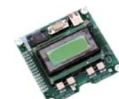
Elevator board Schindler ID.NR.560185 UP000951
