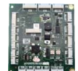
Elevator board Mitsubishi P203728B000G01 UP001103
