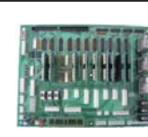
Elevator board Hyundai TCB-3 UP001179
