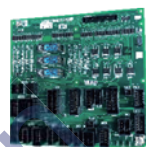
Elevator board Mitsubishi P203736B000G01 UP000035
