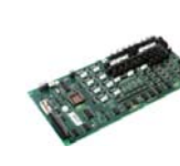
Elevator board ThyssenKrupp MF3 UP000556
