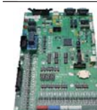
Elevator board Hyundai WBVF Main Board REV1.1 UP001673
