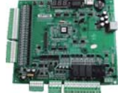
Elevator board Monarch MCTC-MCB-C2 UP000643
