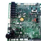
Elevator board ThyssenKrupp UCM CMC4 UP000546
