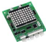
Elevator board Monarch MCTC-HCB-Q2 UP000632
