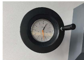
Cutting blade clearance adjustment hand wheel
