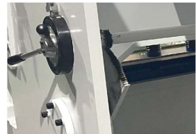
Cutting blade clearance manual adjustment
