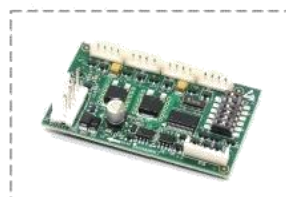
RS14 Otis elevator pcb board
