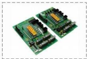
MC24A MC23A Fujitec elevator pcb
