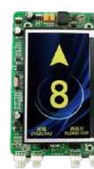
GNL-HD-R-BO-BLU • 4.3 INCH TFT DISPLAY • INSTALL SIZE:118*62MM • FACEPLATE:92*57MM
