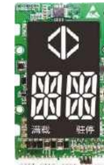
GNL-LED-R • 4.3 INCH LED DISPLAY • INSTALL SIZE:58*40MM • FACEPLATE:76*46MM
