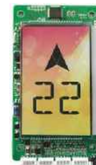
GNL-CBLCD-BO-LIGH • 4.3 INCH LCD DISPLAY • INSTALL SIZE:118*62MM • FACEPLATE:92*57MM
