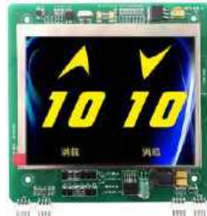
GNL-HD-56-DPLX-BLU • 5.6 INCH HD DUPLEX DISPLAY • INSTALL SIZE:115*120MM • FACEPLATE:87*115MM
