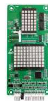
GNL-DOT-R • 4.3 INCH DOT DISPLAY • INSTALL SIZE:134*56MM • FACEPLATE:94*46MM
