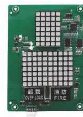
GNL-DOT-64 • 6.4 INCH DOT DISPLAY • INSTALL SIZE:160*105MM • FACEPLATE:140*80MM
