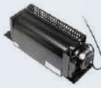
GNL-FB9B-3-11 • FB-9B-3 • Rotate Speed:1250(rpm) • Air Volume:6.5(m³/min) • Power:25(w) • Outlet Size:330X43(mm) • Install size:495X90(mm)
