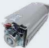
GNL-FB1035B-10 • FB-1035B • Rotate Speed:1250(rpm) • Air Volume:6.5(m³/min) • Power:25(w) • Outlet Size:360X43(mm) • Install size:380X90(mm)
