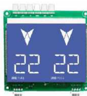
GNL-LCD-64-DPLX • 6.4 INCH DUPLEX LCD DISPLAY • INSTALL SIZE:115*120MM • FACEPLATE:86*115MM
