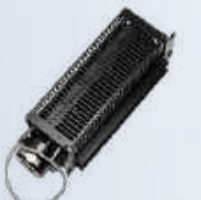
GNL-QF330-22 • QF-330 • Rotate Speed:1700(rpm) • Air Volume:5.5(m³/min) • Power:35(w) • Outlet Size:330X43(mm) • Install size:380X90(mm)
