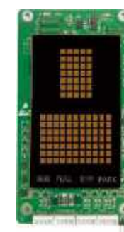
GNL-DOT-NBO • 4.3 INCH DOT DISPLAY • INSTALL SIZE:134*56MM • FACEPLATE:94*46MM
