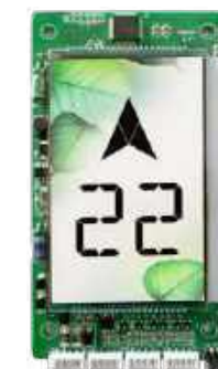
GNL-CBLCD-BO-LEAF • 4.3 INCH LCD DISPLAY • INSTALL SIZE:118*63MM • FACEPLATE:92*58MM
