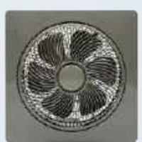
GNL-BAB-24 • BAB • Rotate Speed:1300(rpm) • Air Volume:6.0(m³/min) • Power:45(w) • Install size:300(mm)
