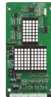
GNL-DOT-R-BO • 4.3 INCH DOT DISPLAY • INSTALL SIZE:94*52MM • FACEPLATE:118*60MM
