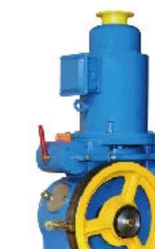
·GF-YJ100 Load:320-408kg Speed:0.5-1.0m/s
